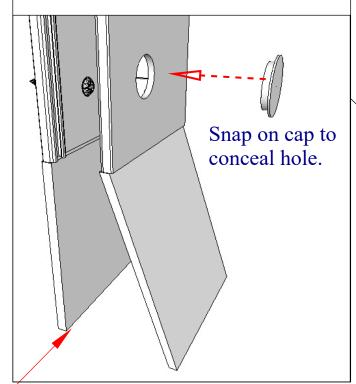
Drill a 3/8" hole in the outside of the side channel to allow access to the screw.
