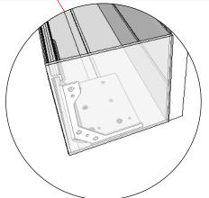
Non Lutron (by special request only) Insert screws through the bracket and pocket as shown below.
