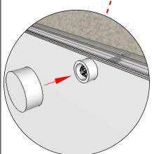
Note - For shades over 96" wide, install the flap support screw in the center of the width of the pocket, 1/8" down from the top of the pocket (through the pocket and into the flap) to support the center. It is important that the screw is no more than 1/8" down from the top and 1.5" long so that it does not damage the fabric. Then snap on the cap to conceal it.
